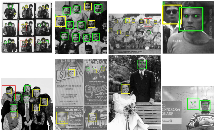
Fig. 1. Detection examples for some CMU database [9] samples. Color indicates the technique used: green means that the eyes were detected, yellow means that they were not detected, and red containing a yellow rectangle means that the local context detector was used. The images have been scaled down to fit the paper size. The size of the images are originally 814 \times 820 , 256 \times 256 , 611 \times 467 and 159 \times 160 respectively in the first row and in the second 500 \times 500 , 539 \times 734 , 336 \times 484 and 258 \times 218 . Obviously for still images there are no detections based on skin color or tracking.
