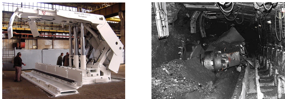
Fig. 1. Shield Supporting system and the Coal-winning shearer working
